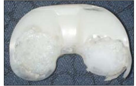
■ Fig 2. Worn out poly due to irradiation in air.
